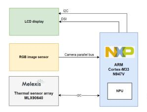
Thermal data is displayed on LCD in heatmap format to allow user to visualize heat distribution of object surface.
